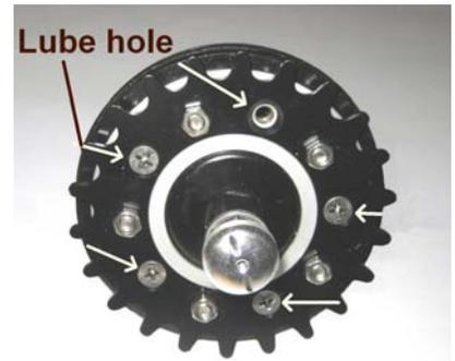
If the **ats-speed-drive** starts running noisily in low gear (when there is no load on the planets) after extended use, this is probably due to a lack of oil on the planet bearings, Insert some lube at the slot screw on the right side. (Please take off one screw of these 5 lube holes only, no need to open all of them !)
