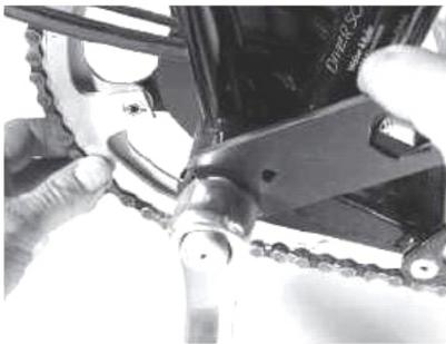
Please note: the adjustment of the gearing play is made at the factory with painstaking accuracy, Do not change the position of the self-locking nut at the left end of the axle without a good reason
